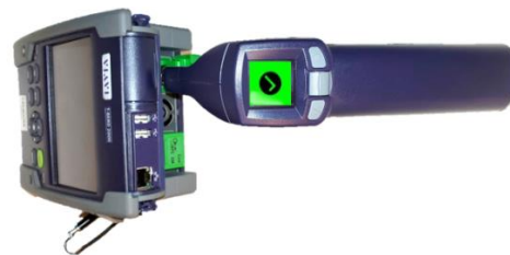
Figure 5: OTDR Port Inspection
