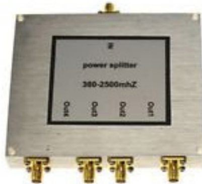
Figure 16. Wideband 4:1 splitter used during commissioning
