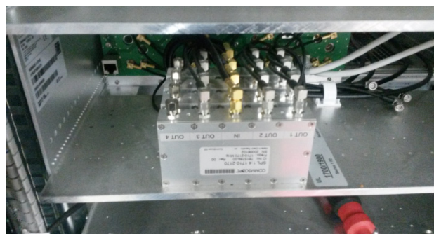
Figure 9. Splitter and combiners
