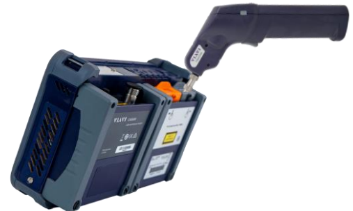
Figure 3: OTDR Port Inspection
