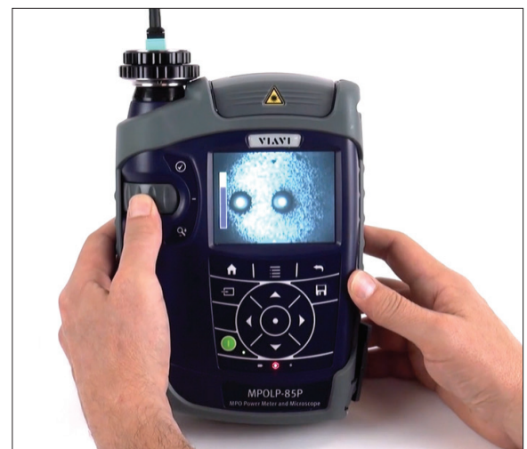
MPO connector inspection with the integrated PCM
